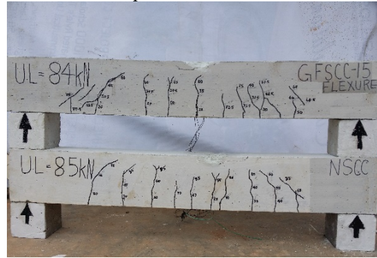
Fig. 5. Crack pattern and failure of NSCC and GFSCC-15 flexure beam specimens
