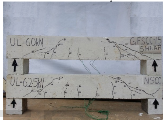
Fig. 6. Crack pattern and failure of NSCC and GFSCC-15 shear beam specimens
